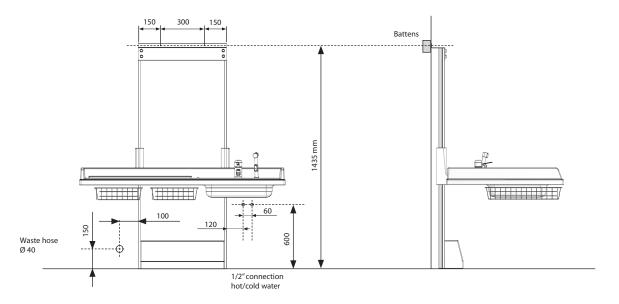
1) Fix the wall stand to the wall by its two upper holes, with the angle brackets turned downwards.
